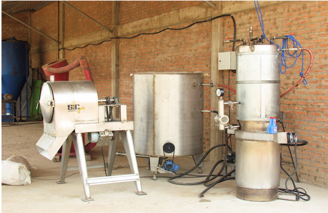
Photo1: right side the gasifier/ water boiler, center the water/ soymilk tank and left the rotating separation sieve.
