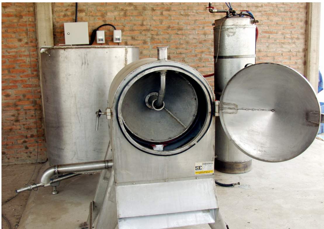
Photo2: Soymilk solids separator with a rotating sieve fed through the center
