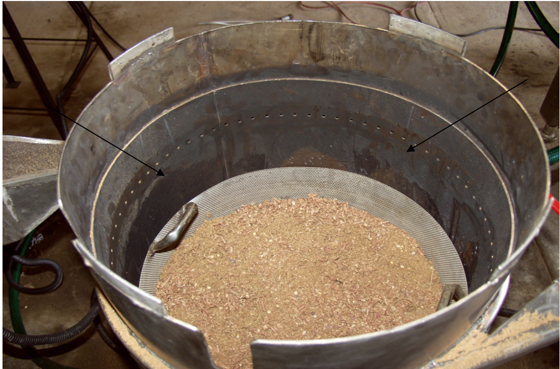
Photo 3: Inside of the gasification part, metal net basket inserted, the arrow points to the air feeding holes for the gas burning zone
