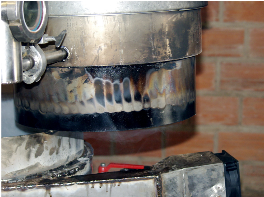
Photo 7: Using wet sawdust at low air feed, to have a good flame distribution indicator, under dry sawdust conditions no blackening visible
